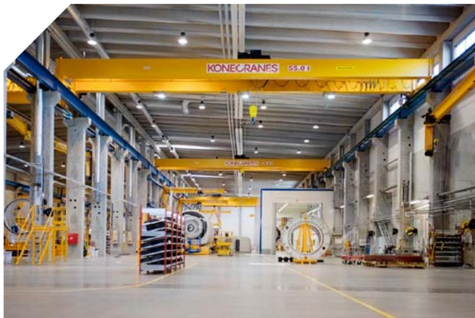
The most important needs for WinWinD were capacity and safety. Because the wind turbine nacelle weighs about 130 tons, and the hub about 30 tons, the lifts constitute a safety issue for personnel and materials. The magnitude of the lifts, on the other hand, required lifting equipment with an extremely effective lifting capacity. Accuracy of the lifts was the most critical factor in the lifting and safety was the highest priority.
